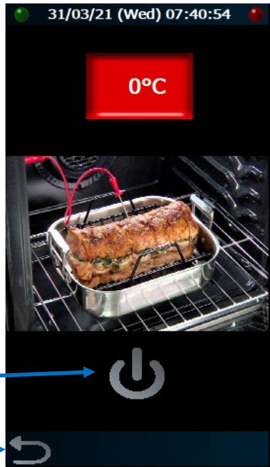
Core temperature cooking uses the temperature in H.A.C.C.P Value on the **Settings Screen** to determine when the food has reached temperature.
