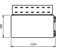
Diagram of the MH9 model with additional tray slide fitted
