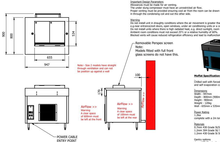
The under slung compressor must have an unrestricted air flow.
