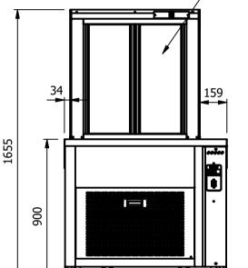
Note:- Size 2 models have straight through ventilation and can not be position up against a wall
