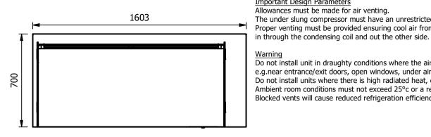
Important Design Parameters Allowances must be made for air venting. The under slung compressor must have an unrestricted air flow. Proper venting must be provided ensuring cool air from the room can be drawn
