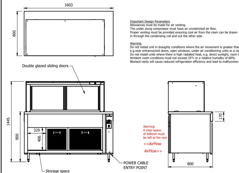
Do not install unit in draughty conditions where the air movement is greater than 0.2mtr/sec. e.g.near entrance/exit doors, open windows, under air conditioning units or a ceiling mounted fan Do not install units where there is high radiated heat, e.g. direct sunlight, room heaters, or bright spot lights.
