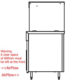
Chilled display with forced air refrigeration and self evaporation condensate system.
