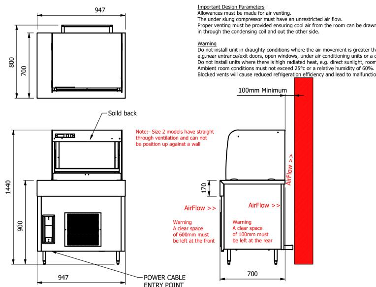
Proper venting must be provided ensuring cool air from the room can be drawn
