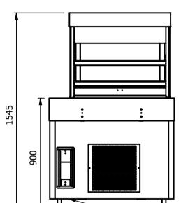
Note:- Size 2 models have straight through ventilation and can not be position up against a wall
