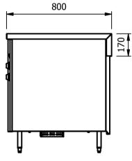
ALL DIMENSIONS IN (mm), TOLERANCE = LINEAR ± 0.5mm, ANGULAR ± 0.5mm (OR AS STATED). ALL SHARP EDGES TO BE REMOVED FROM SHEET METAL PARTS ALL SHEET METAL DIMENSIONS ARE I/S (INSIDE SIZES) (UNLESS OTHERWISE STATED)
