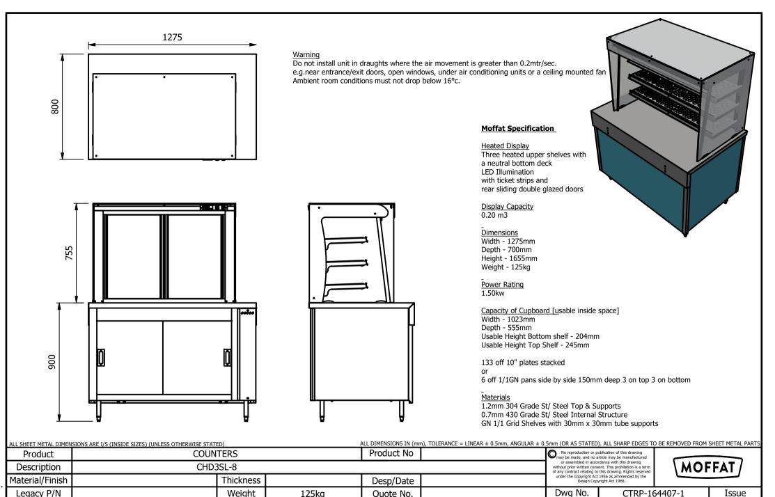
Legacy P/N Weight 125kg Quote No. Client SO Number N/A Drawn By ABB 26/05/2025 **Client Project** Approved By Date E & R MOFFAT LTD, SEABEGS ROAD, BONNYBRIDGE, FK4 2BS, T: +44 (0)1324 812272, E: sales@ermoffat.co.uk, Web: www.ermoffat.co.uk Scale 1:20 Sheet 1/2
