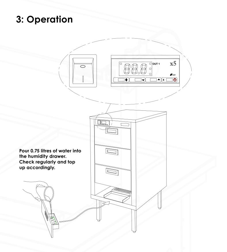
Be careful water may spill from the humidity tray when removing the crumb tray.
