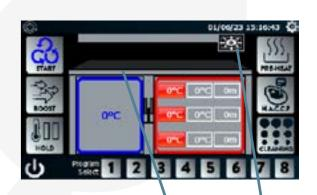
7. When Automatic Hot Top is Off, the hot top can be operated by pressing the hot top on the screen .
