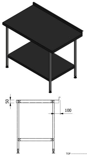
ALL DIMENSIONS IN (mm), TOLERANCE = LINEAR ± 0.5mm, ANGULAR ± 0.5mm (OR AS STATED). ALL SHARP EDGES TO BE REMOVED FROM SHEET METAL PARTS.
