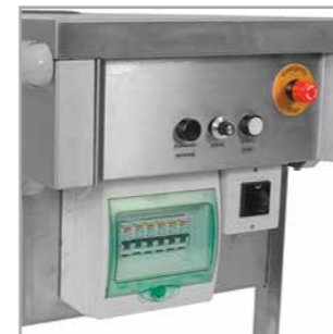
Control panel & splash proof distribution switch board
