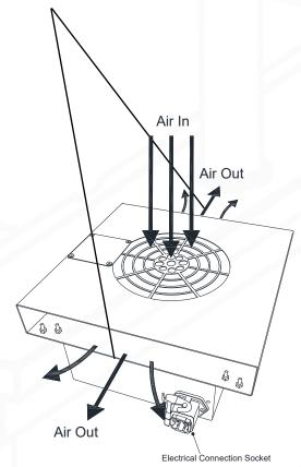
2. Access the plug and socket via the underside of the unit push the locking button on the plug and pull to release
